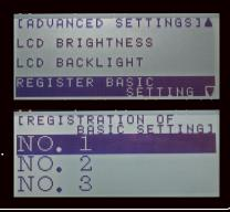
\*In addition to the above functions, you can also set LOW TEMPERATURE MODE/AUTO POWER-OFF/ JUSTIFICATION(LEFT/CENTER/RIGHT FOR NORMAL PRINT MODE and PRINT STYLE OF REPEAT & SEQUENCE.
